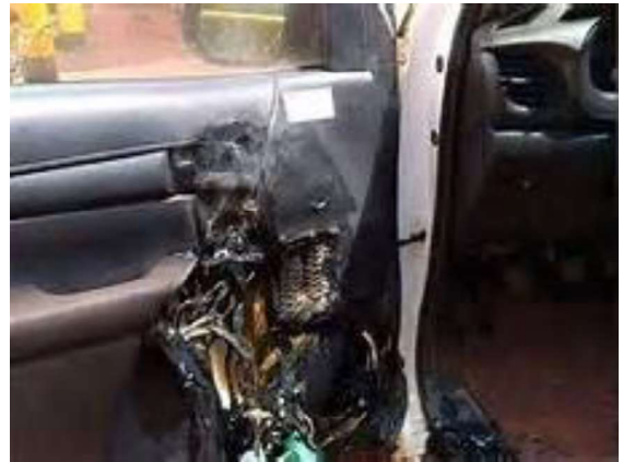
This picture shows damage to a car as result of hand sanitiser fire
